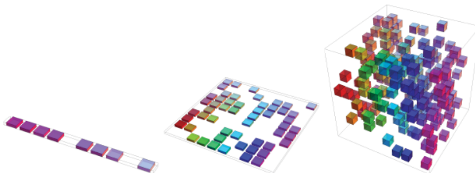
Figure 5.9: As the number of relevant dimensions of the data increases (from left to right), the number of configurations of interest may grow exponentially. ( Left ) In this one-dimensional example, we have one variable for which we only care to distinguish 10 regions of interest. With enough examples falling within each of these regions (each region corresponds to a cell in the illustration), learning algorithms can easily generalize correctly. A straightforward way to generalize is to estimate the value of the target function within each region (and possibly interpolate between neighboring regions). ( Center ) With 2 dimensions (center) it is more difficult to distinguish 10 different values of each variable. We need to keep track of up to 10 \times 10 = 100 regions, and we need at least that many examples to cover all those regions. ( Right ) With 3 dimensions this grows to 10^3 = 1000 regions and at least that many examples. For d dimensions and v values to be distinguished along each axis, we seem to need O(v^d) regions and examples. This is an instance of the curse of dimensionality. Figure graciously provided by Nicolas Chapados.
